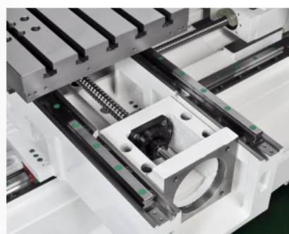
2 linear guide way with 4 slide blocks in X axis
