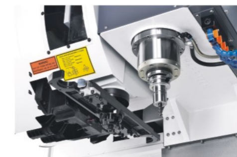
Swing arm ATC and spindle nose
