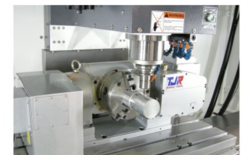
4th axis rotary and with tilting axis
